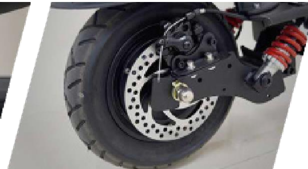
Rear disc brake disc with spring damper
